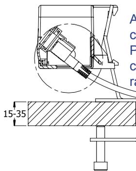
Angled data fascias allow data cabling to pass straight through PULSE-8, ensuring the integrity of cables which have a minimum bend radii (CAT5e, CAT6 etc)
